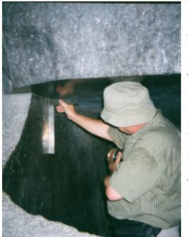
which it sits. The precision square I used was calibrated to .00005 inch (that is 5/100,000 of an inch) using a Jones & Lamson comparitor.
